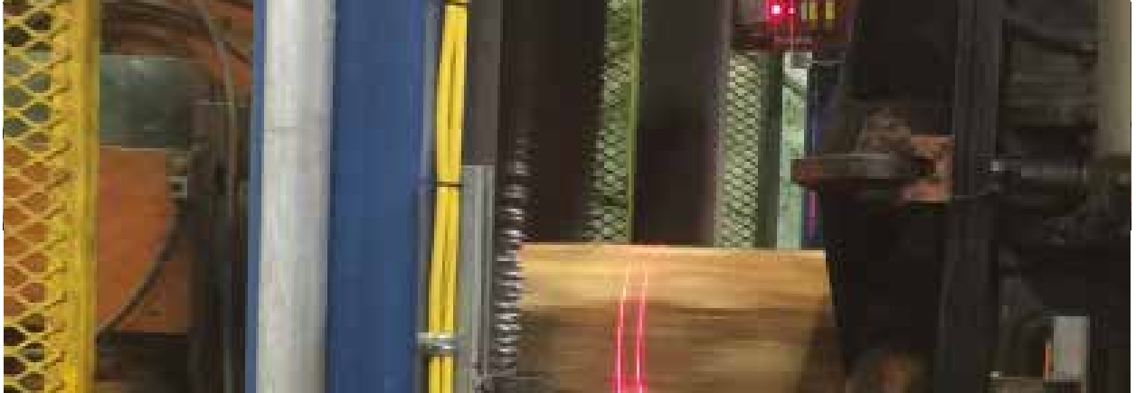
HD laser profile data is captured along the entirety of the piece at a scan rate of 400 Hz.
