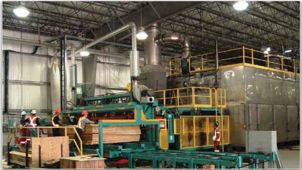
Coe’s veneer dryer technology advanced along with its lathes under Fred’s leadership.
