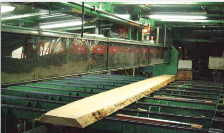
Mill personnel made significant modifications to the scan frame so that it now accommodates the BioLuma 2900L sensors.
