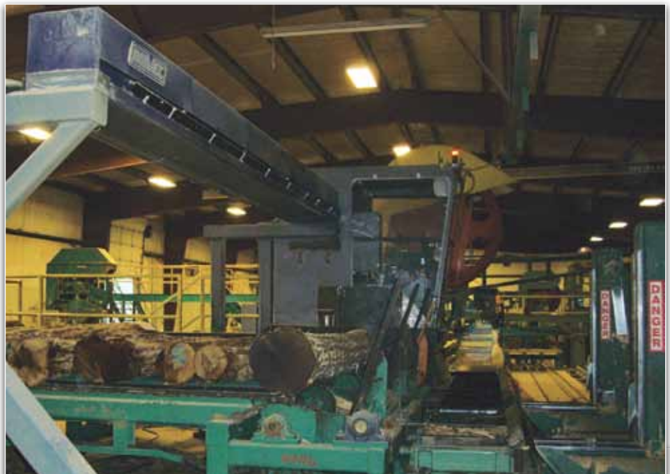
The YieldMaster scanner is positioned above the logs and scans each one after it is loaded and dogged on the carriage.
