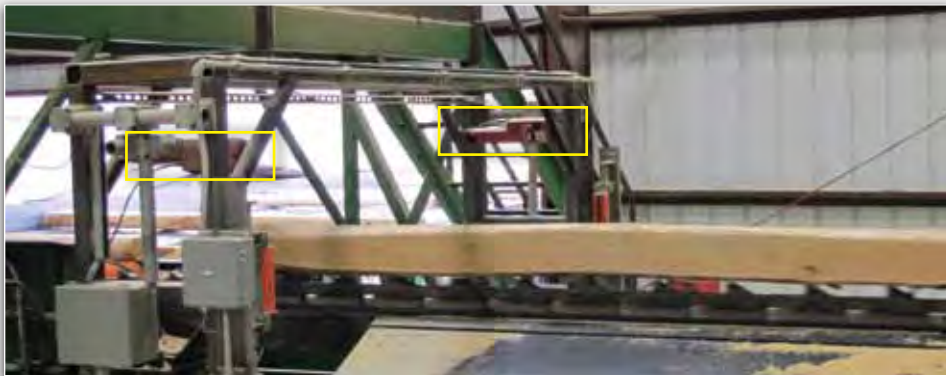
Griffin's SQI system uses 2 Smart TriCam sensors mounted in the log line after the bandmills to scan the cant. Some mills choose to use their spare sensors for this application.
