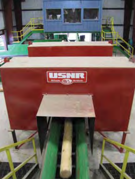
The log is first scanned in a dual zone orientation, for log rotation optimization.
