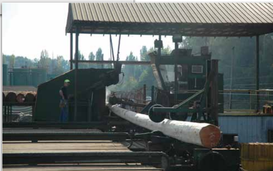
A pole is peeled prior to drying.
