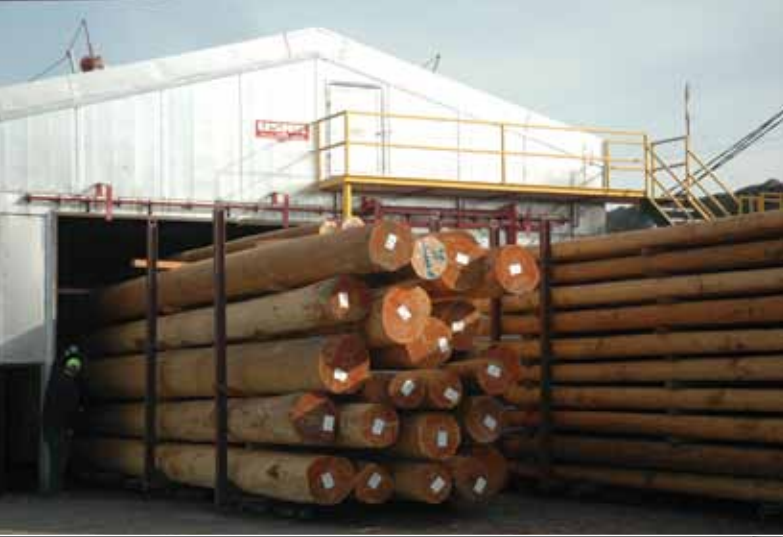
Poles exit the dry end of the kiln once the drying cycle is complete.
