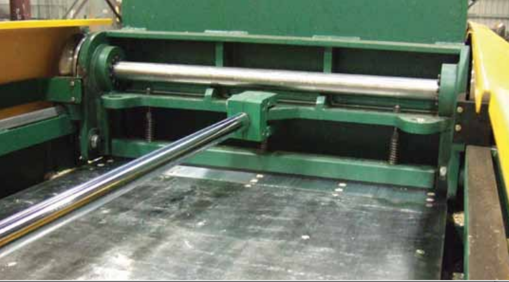
The hopper strokes back and forth via an hydraulic cylinder at a maximum speed of 100 feet/min.
