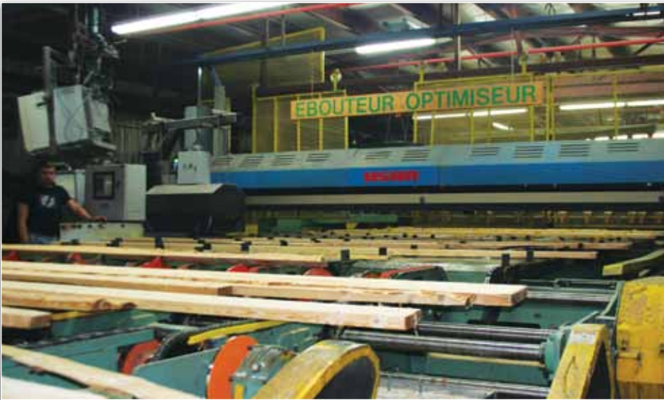
The BioLuma 2900L sensors provide the trimmer optimizer with precisely accurate laser profile measurements, allowing the mill to reduce trim loss and to increase value and recovery.
