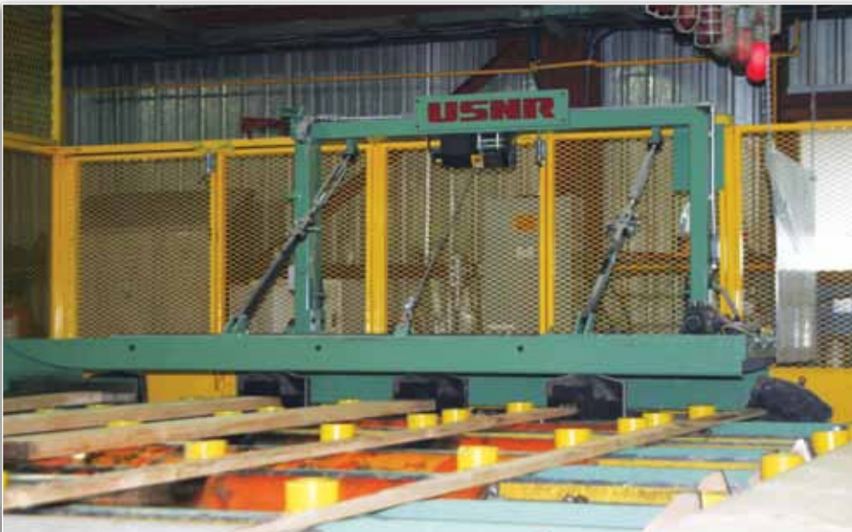
The Multi-Track Fence has become a favorite among lumber producers. It is compact, highly accurate, and easy and cost effective to maintain.
