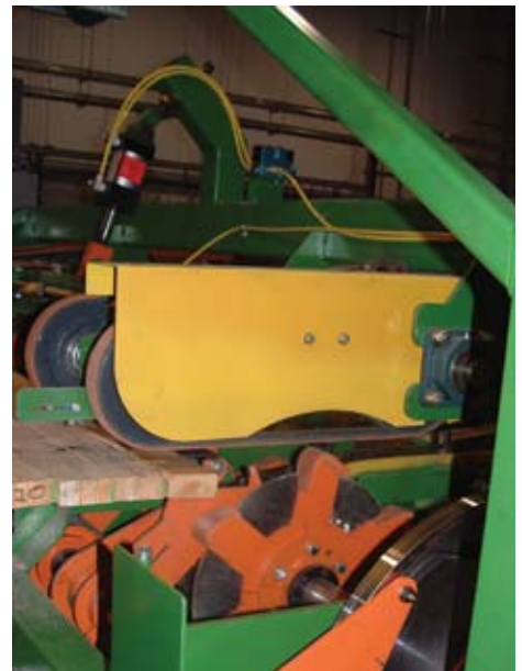
The starwheel shoe enhances positive board feeding.
