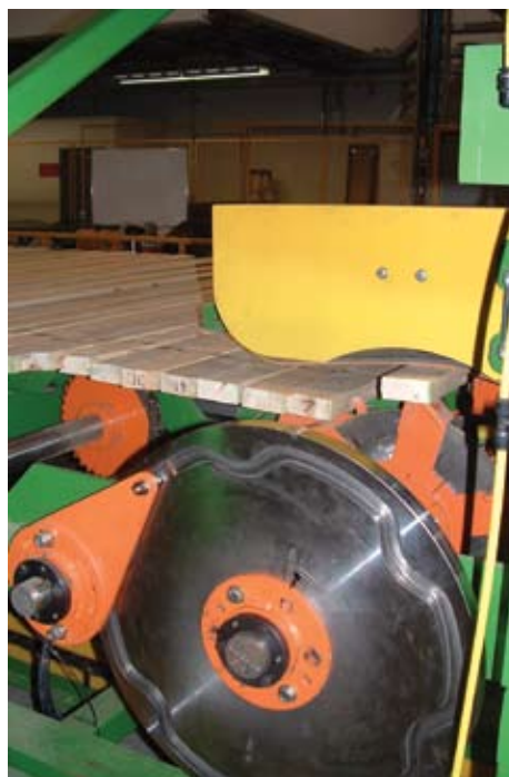
The computer-designed cam raises and lowers the duckers, with minimal wear and maintenance.
