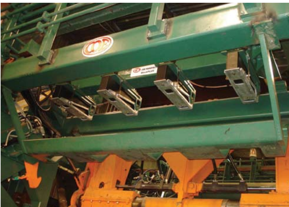
Four 3D laser scanners mounted above, scan the block as it is rotated.
